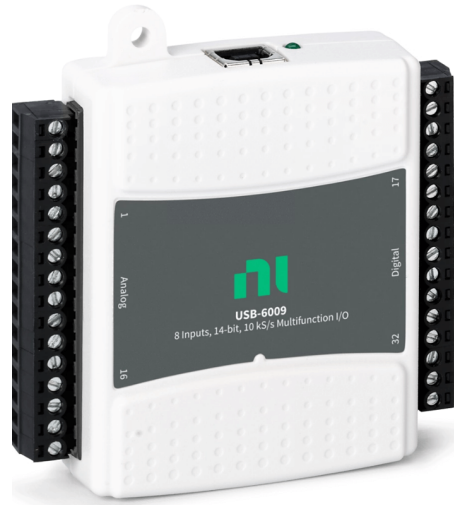
Nidaq (pure connector block, no processing)
